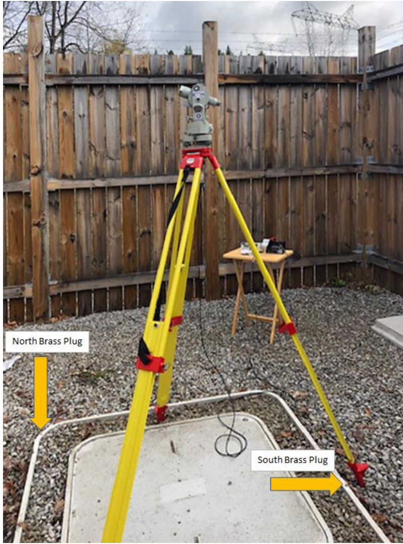
Fig. 7 Sensor Vault with Permanent Azimuth Marks and DIM for Absolute Observations at Essa
