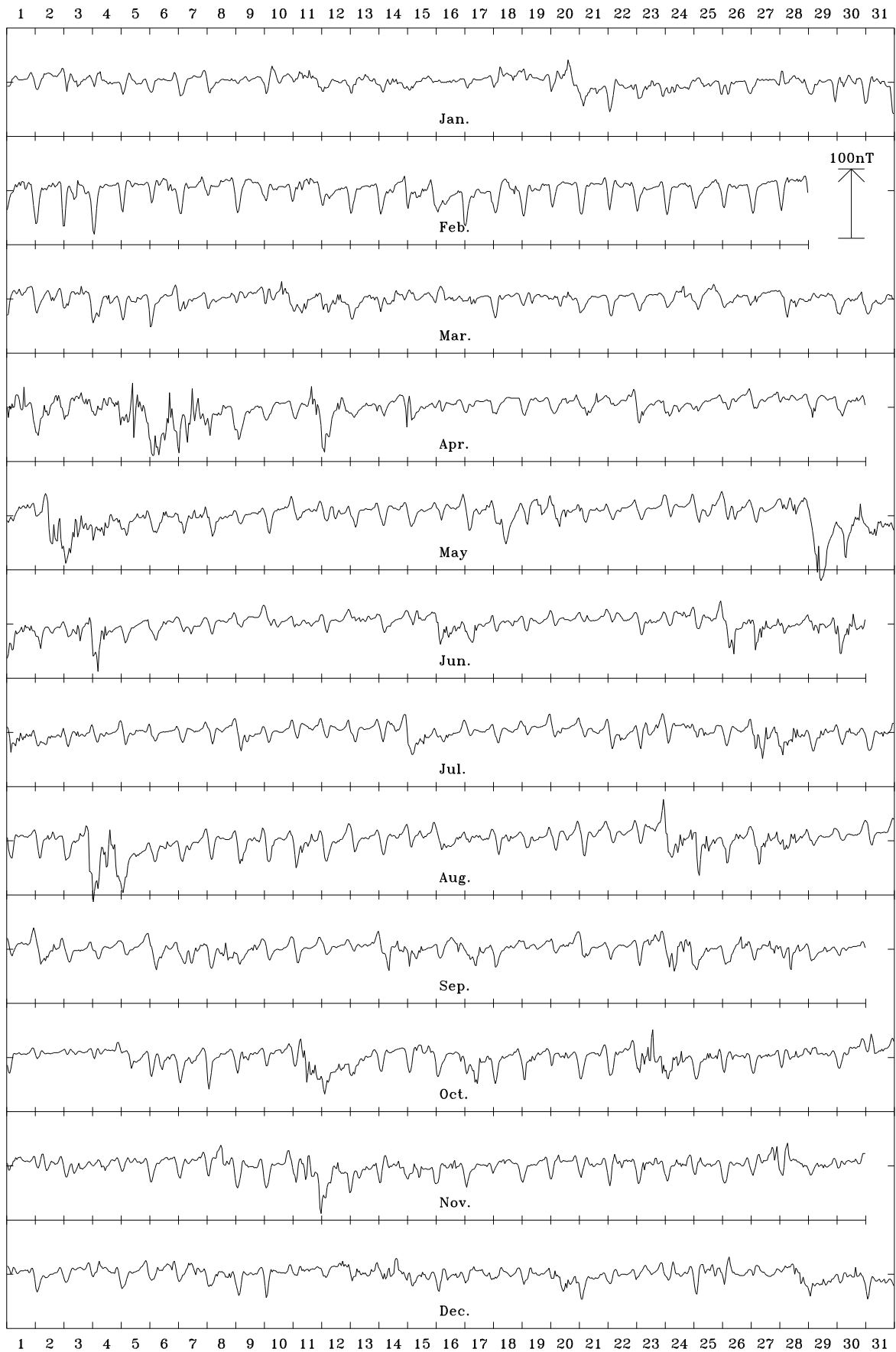
Canberra 2010 North component (X). Scale: 7.5 nT/mm. Mean: 23178 nT
