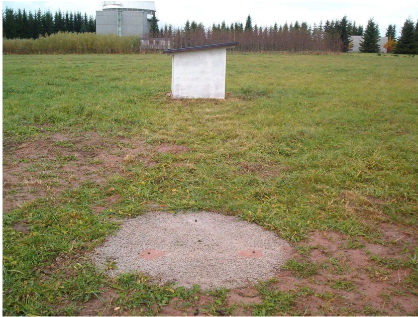
Figure 5: The magnetometer hut at the Tõravere (TAR) observatory in Estonia. A new concrete basement for secular variation measurements in the front.
