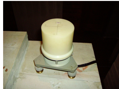
Figure 3: The LEMI-004 magnetometer electronics on the left and the sensor above.
